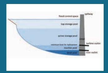
Distribution of reservoir water allocations; a proposed trading approach would allow users to "carry over" unused water as storage credits within a new "top storage" pool; this water could be traded to other users (and spills first in the event that the space is needed for flood control).
