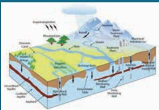
Example of a more sophisticated approach to aquifer management that reflects the active maintenance of multiple values associated with an aquifer through controls on groundwater use, monitoring activities, and active recharge through injection wells, recharge basins, and use of "natural recharge infrastructure" via wetlands and stream flow. Image courtesy of California Department of Water Resources.
